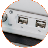
USB Ports on Front and Side for Barcode Scanner and Wi-Fi
