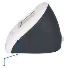
Alternatively, insert AC adapter plug into the power receptacle. Only use AC Adapter supplied by SunTech Medical.
