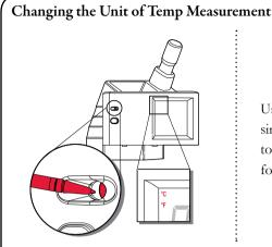
Using the end of a paper clip or similar tool, press the recessed button on the temp module. The icon for the selected unit is displayed.
