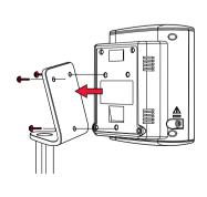
Assemble the mobile stand according to the manufacturer's directions. Using the three thumb screws, secure the rear panel of the BP device to the stand.
