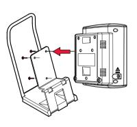
Using the thumb screws, secure the rear panel of the BP device to the stand.
