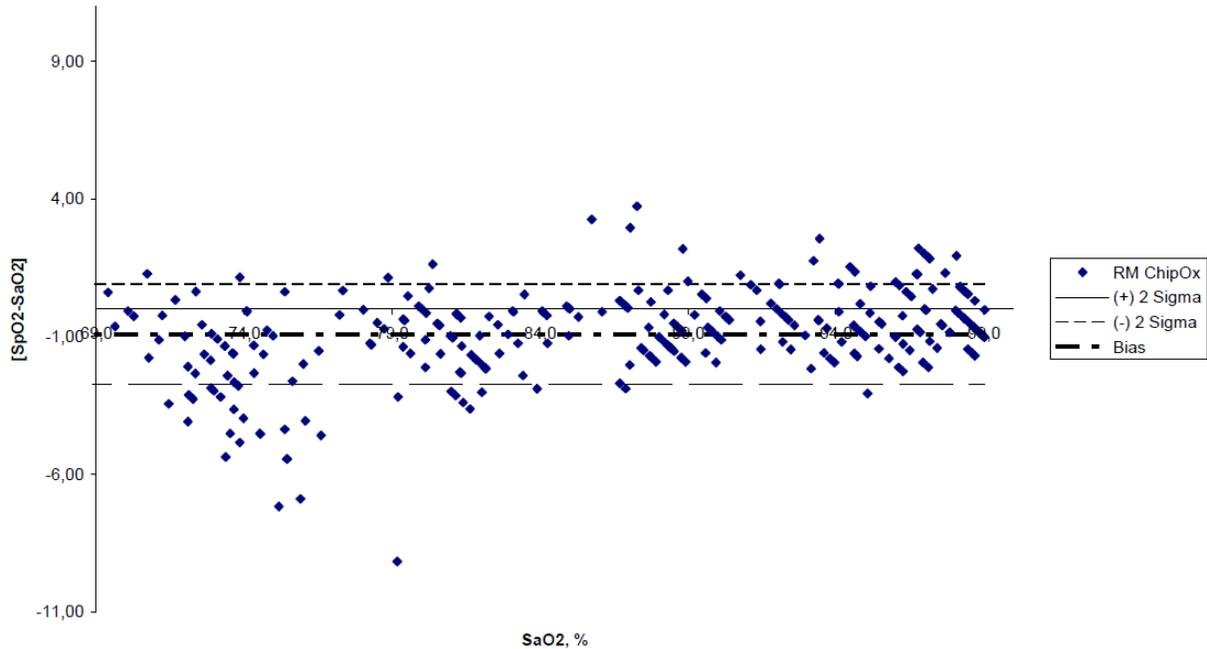
The tested device meets the stated accuracy specification of RMS Error = 1.89% for the range 70% to 100% SaO<sub>2</sub>. The accuracy is not specified below 70% SaO<sub>2</sub>. In addition, here are detailed measured A<sub>RMS</sub> values over the specified discreet ranges:
