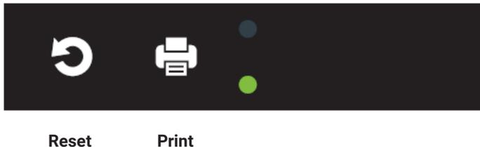
To print the information currently displayed on the CT40 screen, press the print button on the top of the printer (see diagram above).
