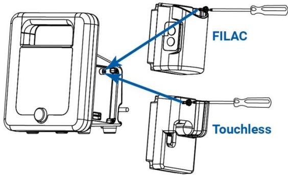
To add a temperature module, attach the module on the right side of the main unit. Fasten with the included Phillips-head screwdriver.
