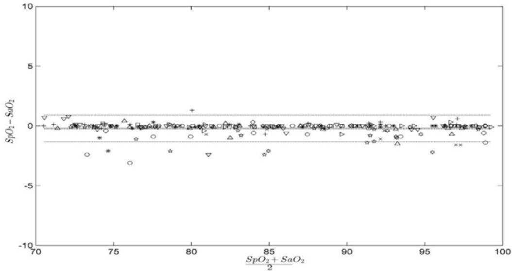
The tested device meets the stated accuracy specification of RMS Error = 2.00% for the range 70% to 100% SaO<sub>2</sub>. The accuracy is not specified below 70% SaO<sub>2</sub>. In addition, here are detailed measured  $A_{RMS}$  values over the specified discreet ranges:
