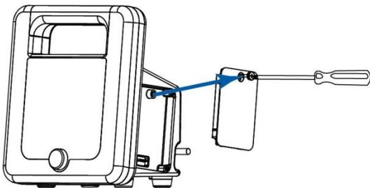
If no temperature module will be added, then attach the right panel of the CT40, using the included Phillips-head screwdriver. This panel will be on the right side, when the screen is facing the user.
