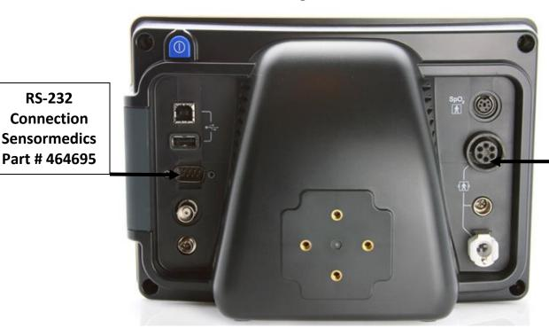
**ECG Trigger** Connection Sensormedics Part # 772539
