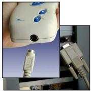
Connect the PC interface cable to the monitor connection at the bottom of the unit.
