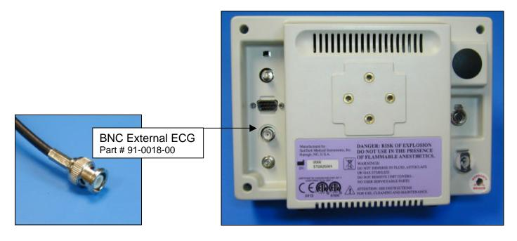
1. Plugging in the ECG trigger cable
